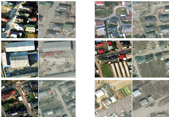
Figure 2. Six samples in the ABCD dataset. Each consists of pre- and post-tsunami patches. The target building is at the center for “washed-away” (left column) and “surviving” (right column).
